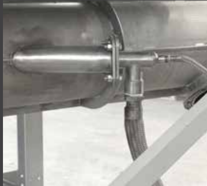
Urea injection lance Low air pressure up to 60 L/h
