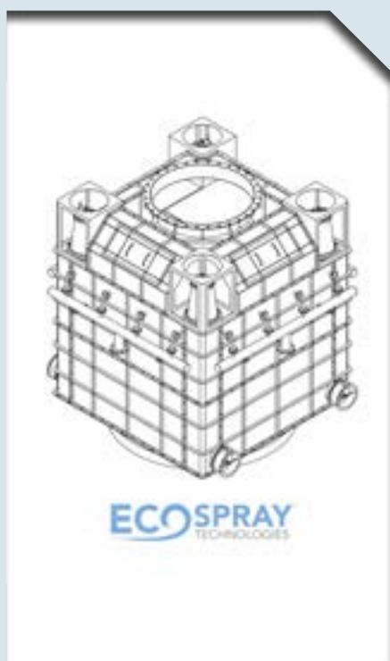
To address those issues, we developed a Wet Electrostatic Precipitator (WESP), with the aim of capturing the remaining dangerous diesel particles (PM2.5 and lower) from the exhaust gas and a good part from condensed matter such as SO<sub>3</sub> created by the gas cooling inside the scrubber.
