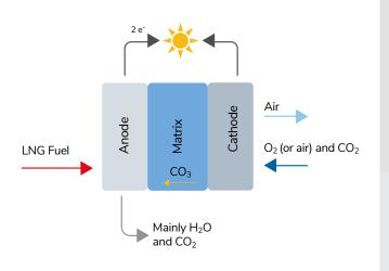
Our new generation of Molten Carbonate Fuel Cells can significantly reduce the ship  $CO_2$  emissions. Several options for the  $CO_2$  storage, onboard and ashore are being studied.
