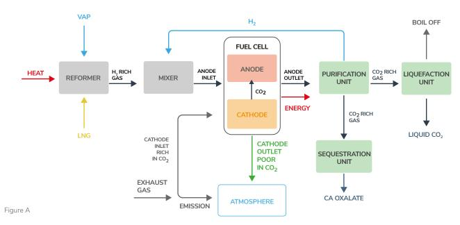
Molten Carbonate Fuel Cells (MCFC) are based on a mixture of carbonate salts as electrolytes. The fuel cell needs to operate a high temperature (approx. 600°C) in order to melt the carbonate salt; only in liquid form the salts are capable, by diffusion, of exchanging carbonate ions, thus working as electrolytes.
