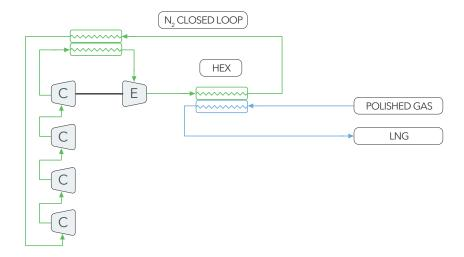
Wet gas (flare & well) liquefaction process
